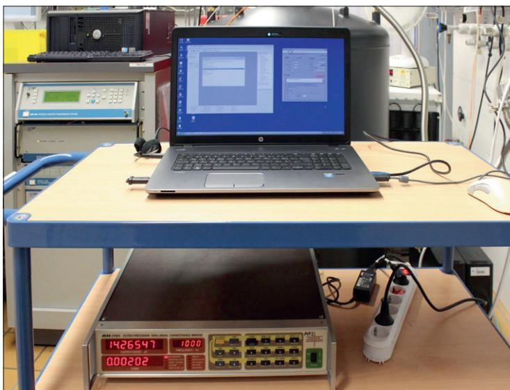
Connect the capacitance measuring bridge by means of a standard GPIB-cable (1) to the PPMS-computer interface and via GPIB-USB-HS converter (2) to your computers USB-interface.
