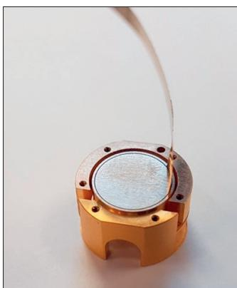
Now the gap between the capacitor plates and its surrounding guard rings can be cleaned by using a very thin and precisely cut metal foil. Use a microscope to check the cleanliness of the dilatometer part. If after cleaning there is still a short circuit in between the plate and the cell body, some very small particles of dirt could be hidden below the capacitor plate. Then the dilatometer part has to be cleaned in an Ultrasonic cleaner.
